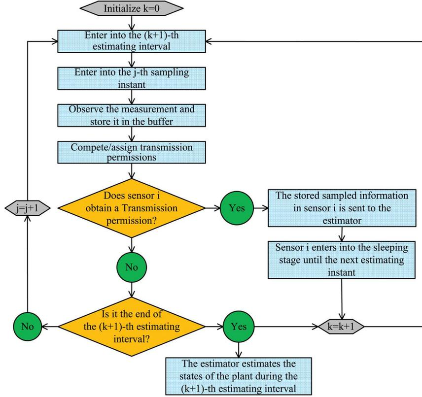
Fig. 2. The architecture of the multi-sensor-based estimation process with competitive transmission.
