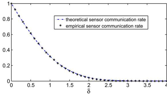
Fig. 4. Sensor communication rate  $\gamma$  versus scheduling parameter  $\delta$ .
